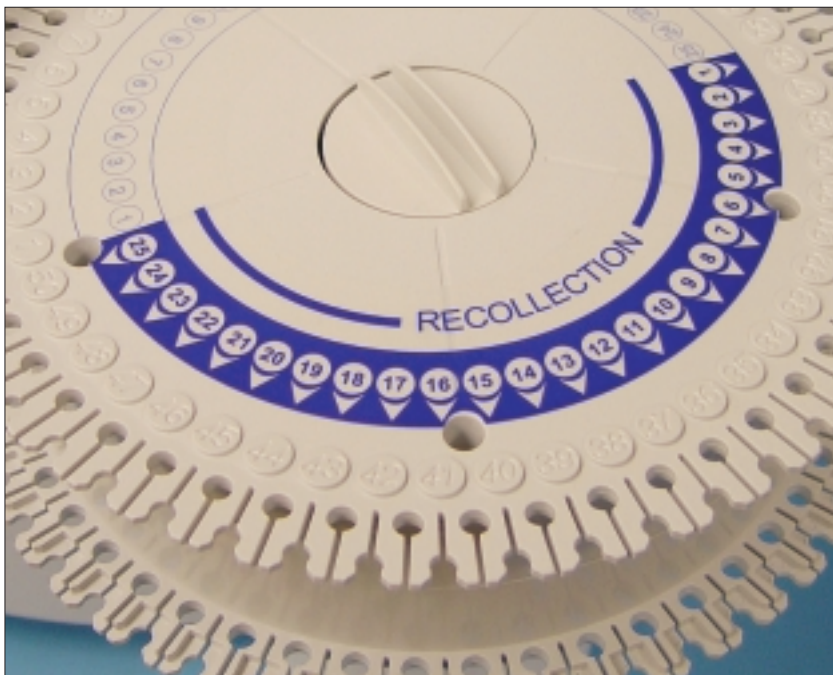
Figure 2. TurboMatrix 650 ATD magazine showing a label associating sample tubes and re-collection tubes.
